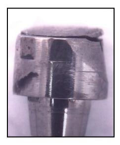
Defect II: Figures 4 and 5 show the effect of abrasion of the cover. Over numerous years, the cover has been worn thin. The lateral defects allow the assumption that an incorrect fit of the cover denture existed. If the abrasion leads to a perforation of the casing, moisture penetrates and comes in contact with the magnet. The subsequent corrosion develops such forces that the cover is literally "blown off" the insert.
