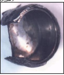
The magnet and the corrosion were removed to allow close scrutiny of the damage. Parts of the cover and of the lateral casing have broken off and the casing has been deformed. The signs of wear and tear as well as the detrimental effects of the corrosion have taken their toll. Additionally, on the cover small cracks are visible and signs of abrasion <sup>9</sup>.
