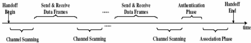
Figure 7: Operation of smooth MAC layer handoff
